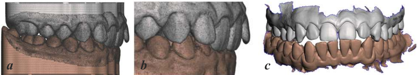
Figure 7. Image of STL files in viewing and editing mesh mixer software. Intraoral scan image. Both images represent STL files, a format used for 3D printing as an exported language by design and planning software. (a) stl files in mesh mixer software, (b) Zoom where you can see the mesh of triangles that compose the file, (c) Intraoral bimaxillary 3d scan view.
