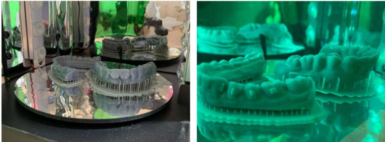
Figure 6. Curing chamber; with rotating plate, adjustable programs for time, light and heat, for post-process 3D printing, walls and mirror-like platform to allow light reflection.
