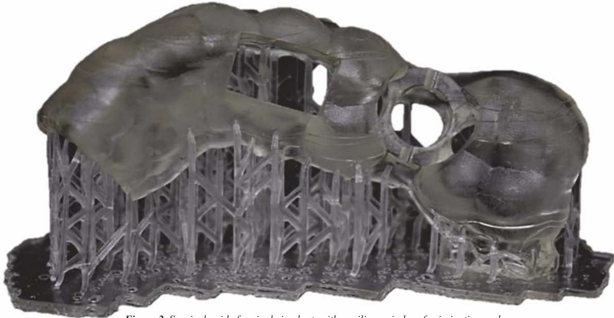
Figure 2. Surgical guide for single implant, with auxiliary window, for irrigation and visualization, printed with biocompatible resin, on Anycubic printer in 1 hour and 30 min. The image shows the base and support pillars placed for printing.
