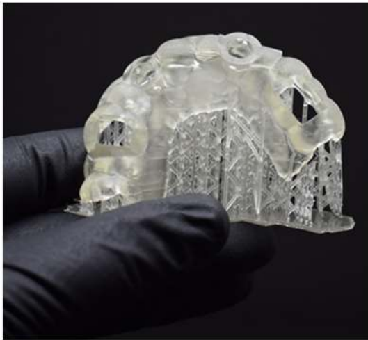
Figure 8. Surgical guide for implants, printed with biocompatible photocurable liquid resin, respecting the principle of devices that are used intraorally with patients. In addition to the precision of details, mechanical properties must be manufactured with ideal materials to be inside the oral cavity. A printed guide is observed prior to the curing process with abutments and support base.
