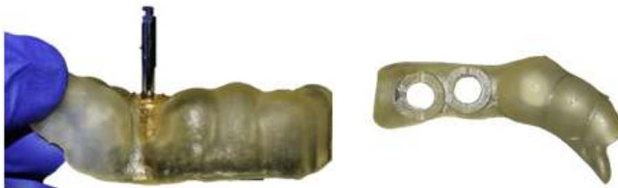
Figure 9. Surgical guide designed for two implants, printed with biocompatible resin, where the precision and accuracy of the diameter of the cylinders is tested prior to clinical use with the patient, to corroborate their measurements with the drill to be used.
