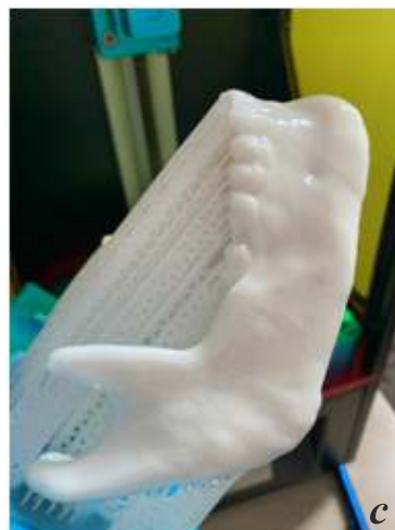
Figure 5. 3D impression of the jaw biomodel for surgery planning is observed in Anycubic printer; with printing size 115Lx65Wx115H with standard white resin. Despite being considered a small desktop printer; it has sufficient dimensions to print larger models like this adult jaw in natural size.
